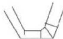
Multiple Cuts for Sharper Angles
